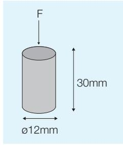
The deformation test is performed at 23° C, 2% deformation/compression, test speed 1 mm/pr. minut in accordance with ISO 604
