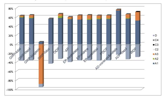
Figure 4: Environmental profile of the LARCORE® A2 panel 14 mm 1.0/1.0
