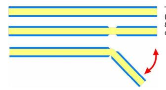
The sheets are also functionally tested by RWTÜV in a broad temperature range. After 80.000 folding movements no deterioration could be observed.
