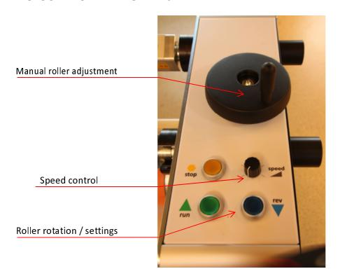
**Roller rotation** – the lower roller is driven by an electric motor. With the EcoLam, the revolutions can be controlled continuously in the range from 0 to 4 m/min.
