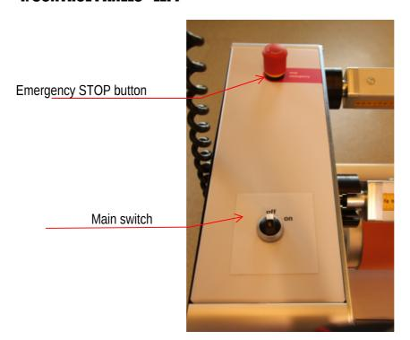
**Emergency STOP button** – If the emergency STOP button is activated, the machine switches off completely. Depending on the circumstances, you can switch the machine on again. The emergency stop switch is deactivated by turning (or pressing - depending on the system used).
