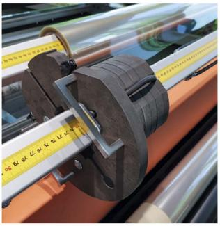
Adapter for holding 150 mm thick industrial cores. The set consists of two adapters, suitable for all 1.650 mm NESCHEN laminators.
