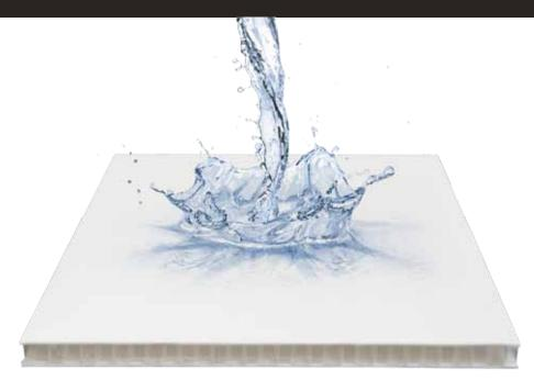
Ultra Board Polyprop utilises Ultra Board structural honeycomb as the core material, which is made from 100% polypropylene. Polyprop Board facings are made from 100% polypropylene, and have a bright white, smooth and glossy surface. The polypropylene is resistant to water and most oils, greases and chemical products. The board is corona treated to enable it to receive ink.
