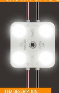
Crown OPTO STELLAR series modules are designed to illuminate huge depth letters and lightboxes. S4 module application is ranging from 140 to 300 mm in depth. These modules come with L70 100 000 h lifetime for 6500K and L70 50,000 h for other colours, granting 5 years warranty. Crown OPTO STELLAR — a great option for projects when economical, although a quality solution is needed.
