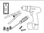
Tools reguired. Wires, wire strippers, drill, screwdriver, screws, surface cleaner, wire connectors and end caps.
