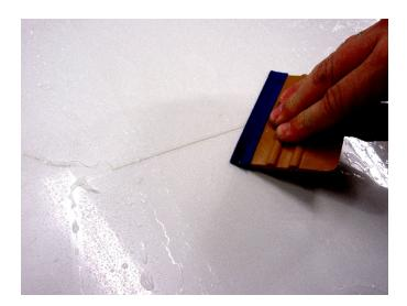
To remove air bubbles, press the film onto the Knifeless Tape again with your finger.
