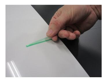
Press thumb firmly on folded edge, covering at least 1 cm tape. Firmly grasp the end of the tape with your thumb and index finger. Start with your two thumbs 1 cm apart. Bring thumbs together and give the tape a quick snap, breaking the carrier tape and exposing the filament (line).
