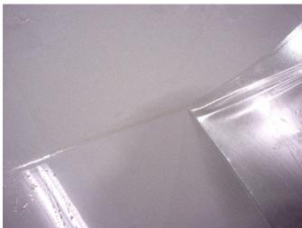
Then remove the carrier tape from under the film while wetting the substrate under the film. Assure that the carrier tape is completely removed without residuals.
