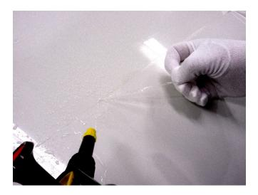
Apply the film edge to the substrate and re-press the film edge with pressure.
