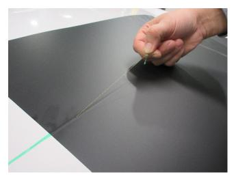
After cutting is finished, remove the excess film and the carrier tape from under the film. Please note that after cutting the carrier tape has split in two tapes. Both tapes need to be removed completely without residuals.
